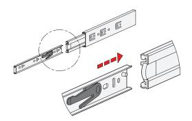
Type F has additionally a detach function through which the extension slides can be completely separated from one another in the area of the middle and inner slide. This feature not only facilitates mounting. It also allows the extension to be quickly removed, for example, when frequent maintenance work is performed on the components located behind.
